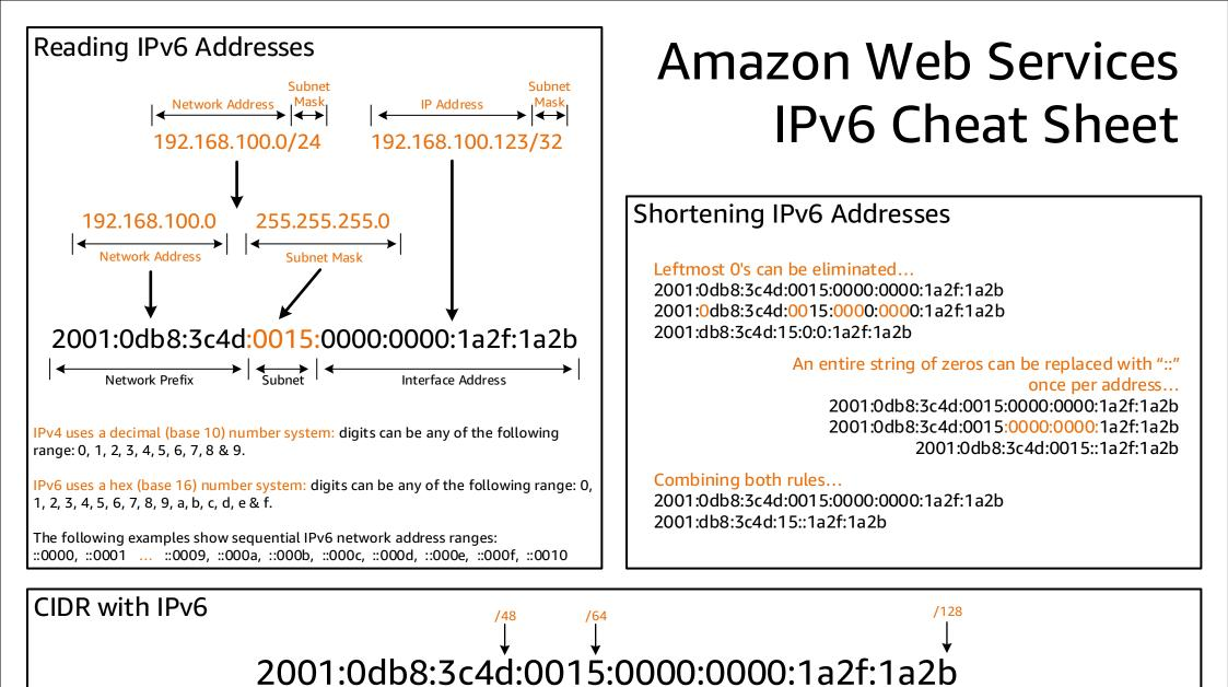
Classless Inter-Domain Routing (CIDR) with IPv6 is similar to IPv4, with a network identifier being followed by a suffix (e.g. /64) indicating the number of bits for the network prefix.
