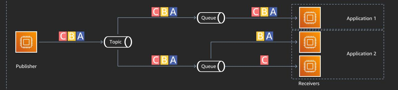
Allows fan-out and receiver scale-out at the same time
