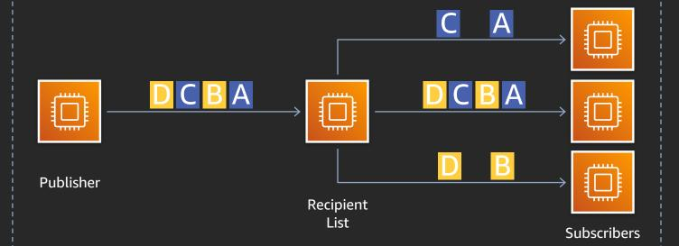
Send only a relevant subset of messages to a subscriber Controlled by publisher or separate component Potentially adds coupling
