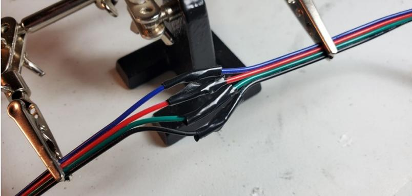
6. Tape all connections together with electrical tape
