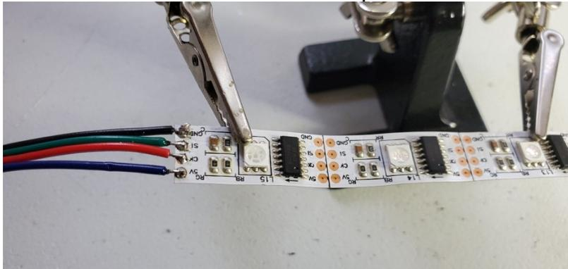
Solder **GND** to the black wire and keep the same order of the wires until you end up soldering **5V** to the blue wire.
