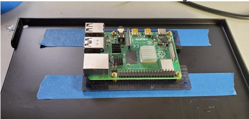
Position the pi on the mic shelf where you would like it to main once mounted. Applying a masking tape or painters tape on the shelf will help you mark where the holes should be.
