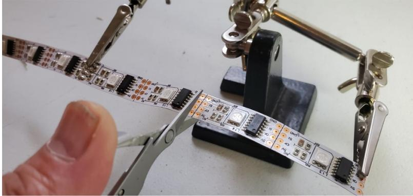
Cut cleanly along the line between the copper leads.
