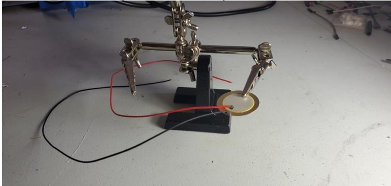
The wires that come with the piezo sensor are quite flimsy. We found that after some moderate use of the drums, the wires fell off the sensors. Resoldering with a heavier gauge wire fixes the problem.
