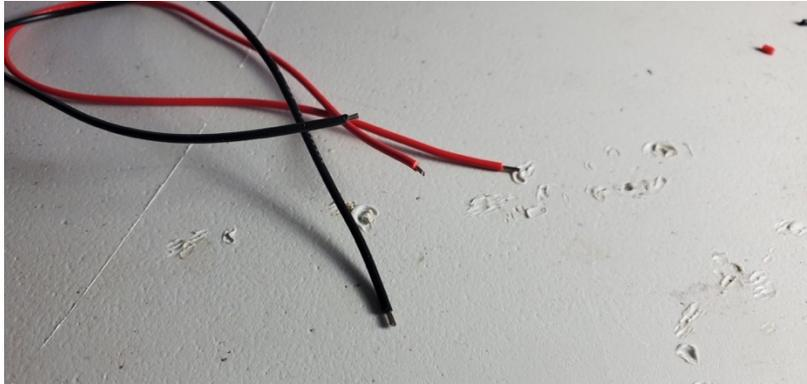
d. Solder extension wires to the piezo sensor
