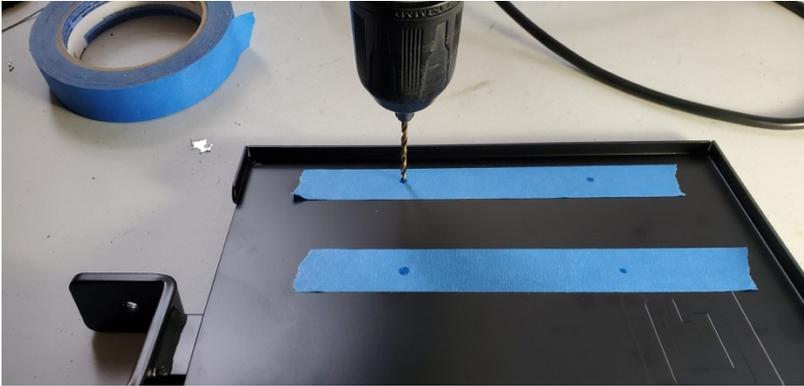
Remove the tape after drilling to see 4 cleanly drilled and well placed holes.
