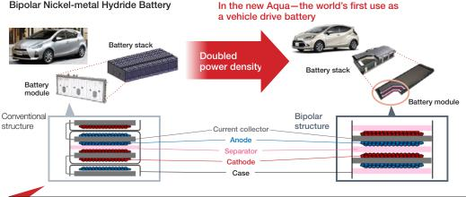
Taking up the challenge of innovating battery structure for more powerful acceleration Power density doubled from the conventional batteries for the Aqua
