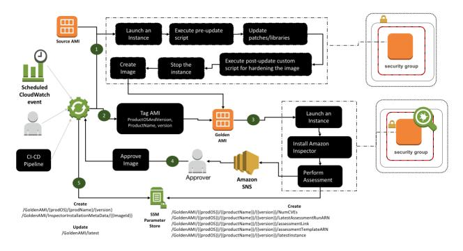
You can trigger the golden AMI creation process in multiple ways. The process may take approximately 30 minutes to 1.5 hours depending upon the available number of updates and scripts executed on the AMI. You can either schedule it to run periodically OR trigger it manually OR trigger it at the end of your CI-CD pipeline.
