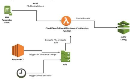
The rule triggers an AWS Lambda function which reads the list of active AMIs from a parameter in the SSM parameter store and marks any instance that has an AMI-ID that does not match with any of the active golden AMIs, as non-compliant. The AWS Config rule gets evaluated on following occasions:
