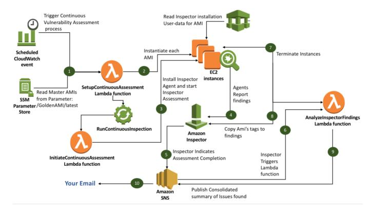
A scheduled CloudWatch Events event triggers the SetupContinuousAssessment AWS Lambda function, which starts the security assessment of your golden AMIs. The SetupContinuousAssessment Lambda function reads a parameter with the key as /GoldenAMI/latest stored in the AWS Systems Manager (Systems Manager) Parameter Store. This parameter contains the comma-separated list of active golden AMIs.
