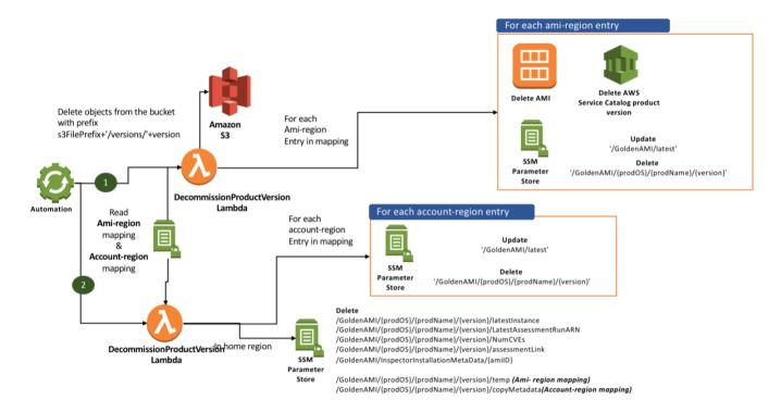
The automation will remove all traces of the specified version including the AMI, copies of the AMI in other regions, and all parameters created in the master as well as the child account. It also deletes the AWS Service Catalog product/provisioning artifact. The process does retain the Inspector assessment result for future reference.
